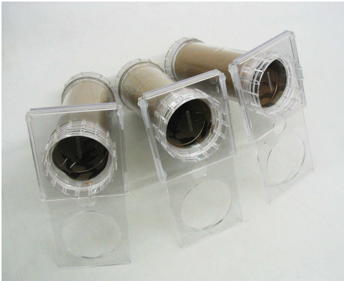
Fig. 1: Standard-WHO-Tubes . The textile sample is inserted into the plastic tube. The transfer tube is not shown (see the Appendix section for further information).
